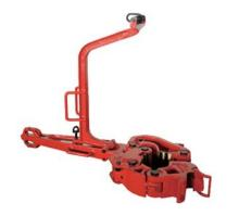
The type SDD manual tong is designed for make-up and break-up of pipe connections with torque capacity up to 100,000 lbs/ft. It can handle OD size from 4-1/2" to 17" by changing out of lug jaw and hinge jaw. The products are designed and manufactured in accordance to API Spec 7K.
