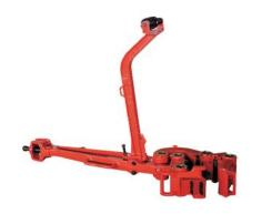
The type B manual tong is designed for make-up and break-up of pipe connections with torque capacity up to 55,000 lbs/ft. It can handle OD size from 3-1/2" to 13-3/8" by changing out of lug jaw. This tong can be extended to handle from 13-3/8" OD - 36" OD casing by using casing head assembly with torque capacity of 50,000 lbs/ft. The products are designed and manufactured in accordance to API Spec 7K.
