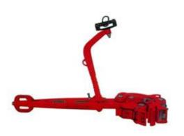
The type DB manual tong is designed for make-up and break-up of pipe connections with torque capacity up to 65,000 lbs/ft. It can handle OD size from 3-1/2" to 17" by changing out of lug jaw and hinge jaw. The products are designed and manufactured in accordance to API Spec 7K.
