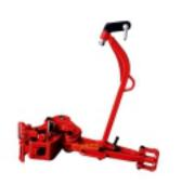
The type LF manual tong is designed for make-up and break-up of pipe connections with torque capacity up to 16,000 lbs/ft. It can handle OD size from 2-3/8" to 7" by changing out of lug jaw. The products are designed and manufactured in accordance to API Spec 7K.
